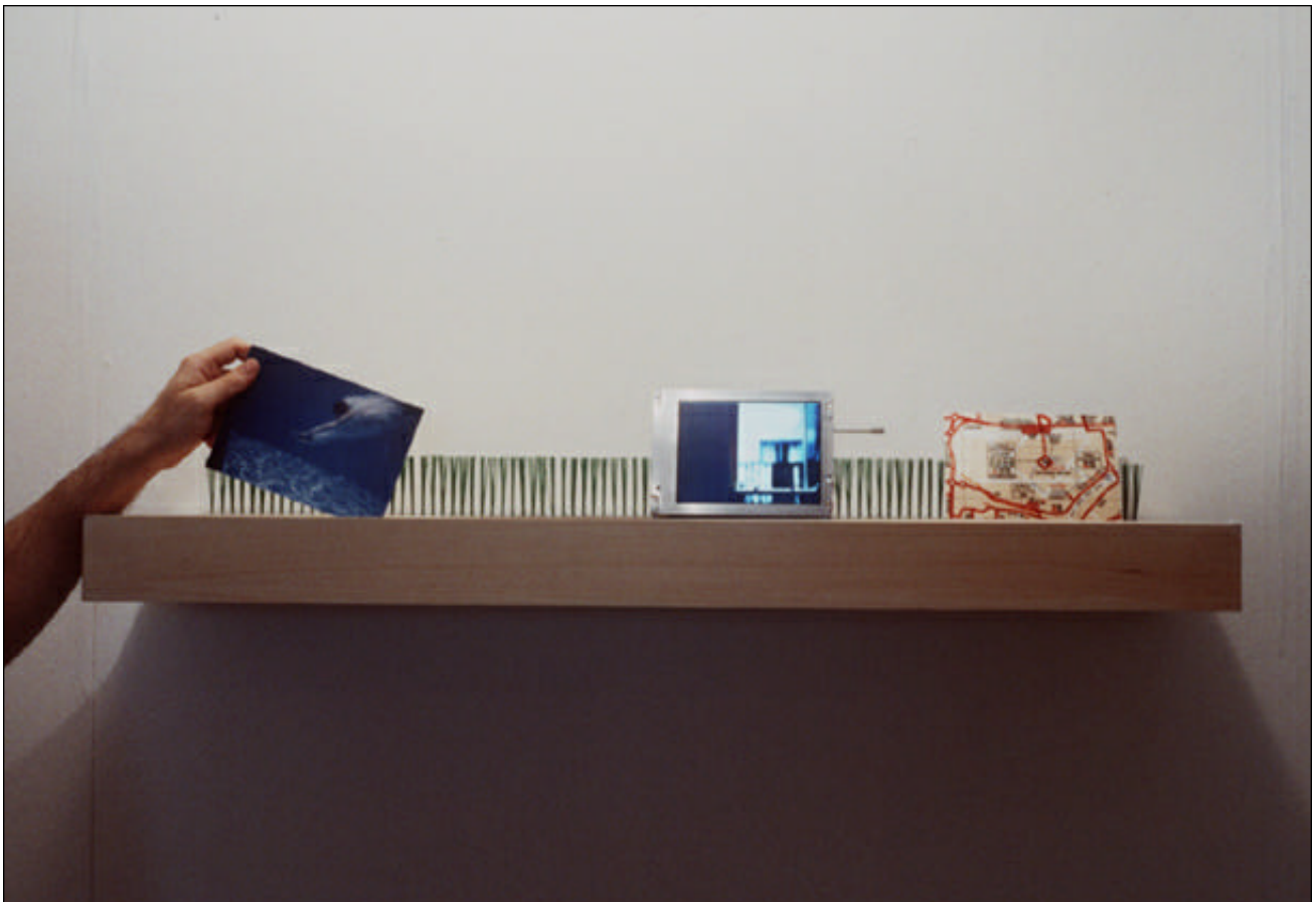
Figure 13. Placing a card in the shelf displays the same image on the small LCD screen and plays its sound simultaneously.
